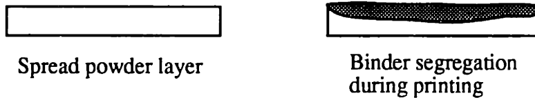
Figure 5: Segregation due to slip casting of the printed slurries (26 vol%) on the SD granule powder bed.
