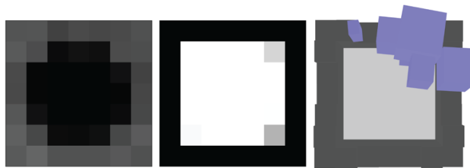
Figure 6.1 Activation of zero latent vector z_0 . Left: obstructions heightmap, where black is zero and white is the maximum height. Center: plot shape, where white indicates buildable plot. Right: complete rendered sample with obstructions in gray, plot shape in light gray, and geometries in blue.
