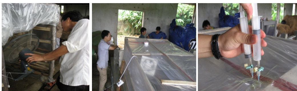
Photo 2. Gas collection for CO 2 and CH 4 determination
