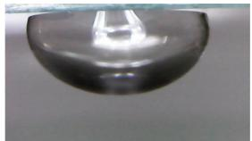
*Figure 1.* Water droplet image on OTS-treated glass slide captured using picture function of Koolertron microscope.
