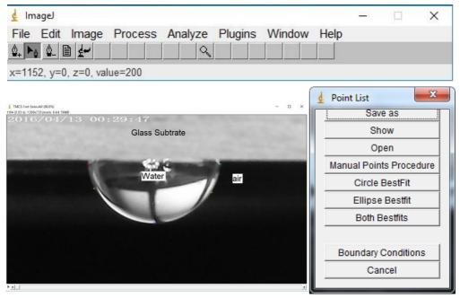
*Figure 3.* Points picking on water droplet
