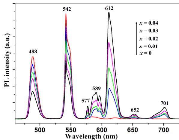
**Figure 5.** Emission spectra of  $\text{YAB}:0.02\text{Tb}^{3+}, \text{xEu}^{3+}$  polycrystalline
