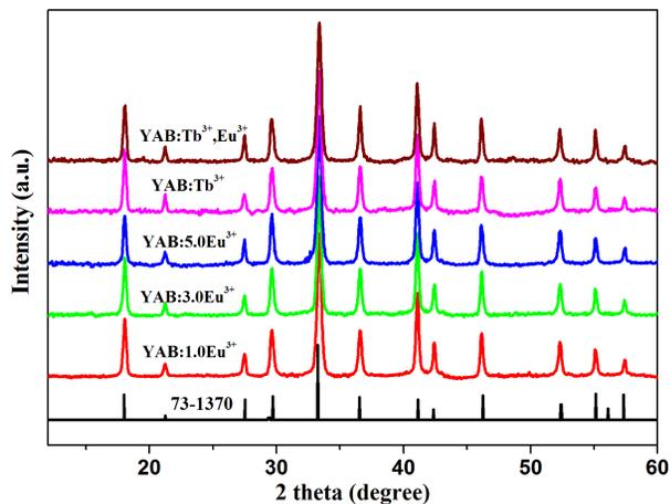
**Figure 1.** XRD patterns of the YAB:RE<sup>3+</sup> polycrystalline
