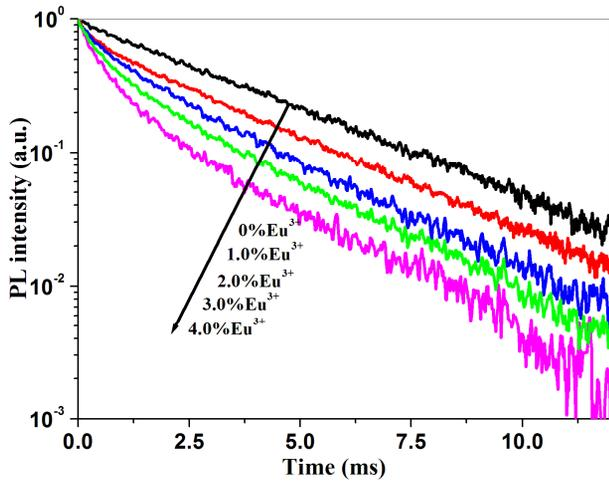
**Figure 6.** Decay curves of  $Tb^{3+}:^5D_4$  level in  $YAB:0.01Tb^{3+},xEu^{3+}$  ( $x = 0.01, 0.02, 0.03$  and  $0.04$ ).
