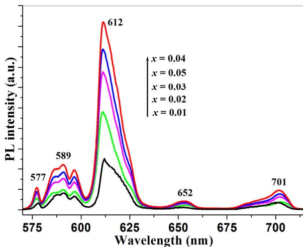
**Figure 3.** Emission spectra of  $\text{YAB}:\text{xEu}^{3+}$  polycrystalline ( $x = 0.01, 0.02, 0.03, 0.04$  and  $0.05$ ).
