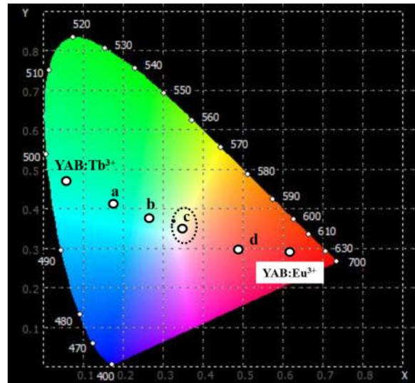
**Figure 4.** CIE Chromatic coordinates diagram of  $\text{YAB}:\text{Tb}^{3+}$ ,  $\text{YAB}:\text{Eu}^{3+}$  and  $\text{YAB}:0.02\text{Tb}^{3+}, \text{xEu}^{3+}$  where  $x = 0.01$  (a),  $0.02$  (b),  $0.03$  (c) and  $0.04$  (d).
