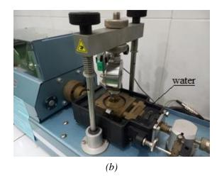
Figure 5. The samples are compacted and then saturated (a) before the shear test (b).
