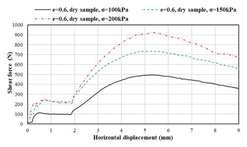
Figure 6. Relationship of shear force and horizontal displacement (dry sample, void ratio e = 0.6, shearing rate 0.25 mm/min).
