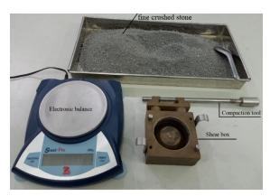
Figure 2. Fine crushed stone at the quarry in Phu Ly - Ha Nam and experiment tools.
