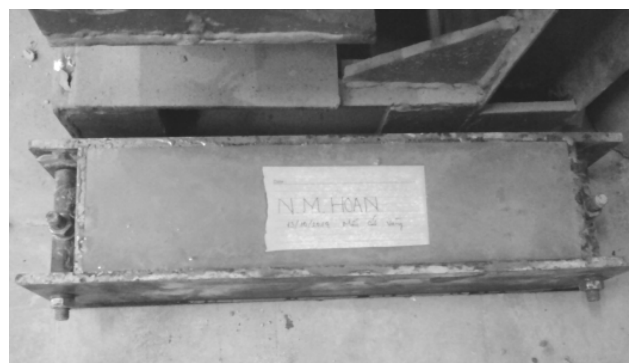
Figure 5. Prismatic specimens for the flexural test
