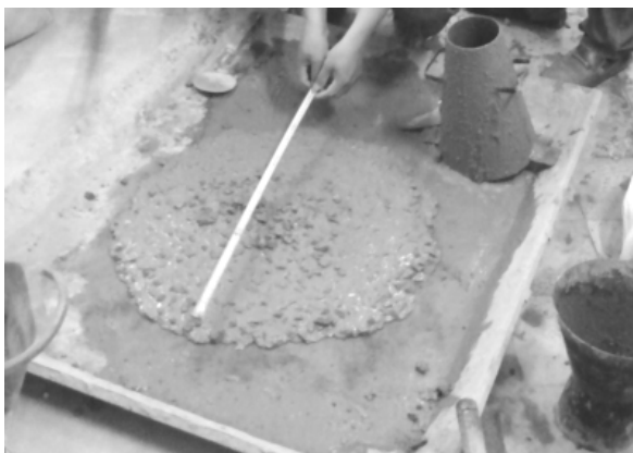
Figure 3. Determination of slump flow value
